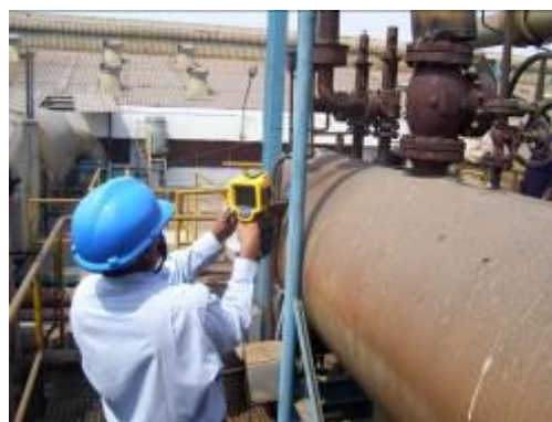
Figure 37: Using Thermal Imaging Camera in a Steam System Assessment
