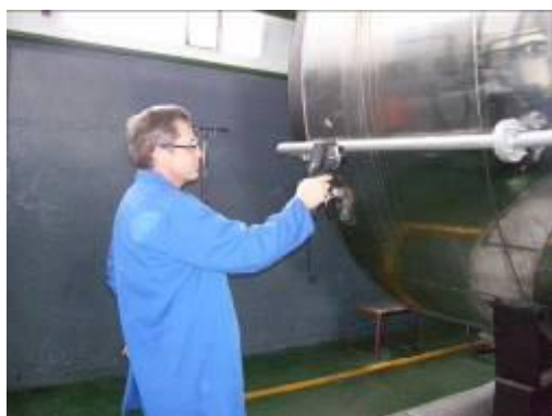
Figure 37: Using Thermal Imaging Camera in a Steam System Assessment
