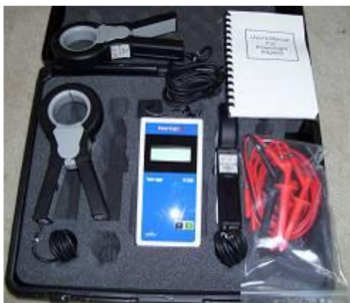
Figure 41: Portable Power meter for use in a Steam System Assessment
