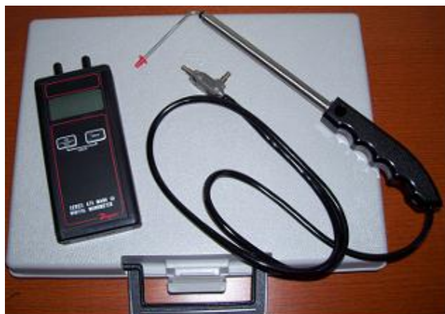
Figure 39: Pitot Tubes (and Digital Manometer) used in a Steam System Assessment
