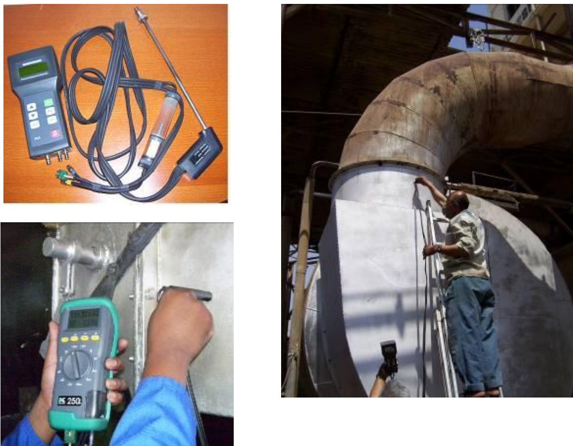
Figure 40: Use of Stack Gas Analyzers in a Steam System Assessment
